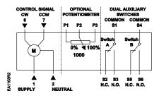
0 to 10 Vdc, GCA16x, 24 Vac/dc; 2 to 10 Vdc, GCA15x, 24 Vac/dc:
